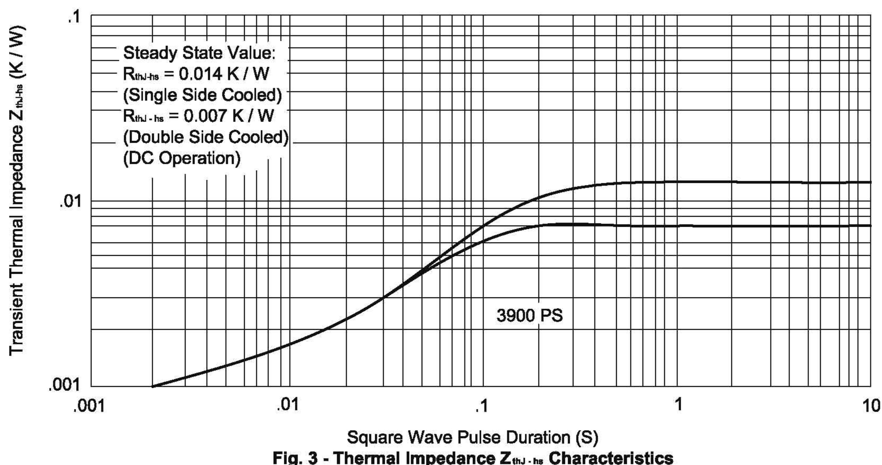
Fig. 3 - Thermal Impedance  $Z_{thJ-hs}$  Characteristics
