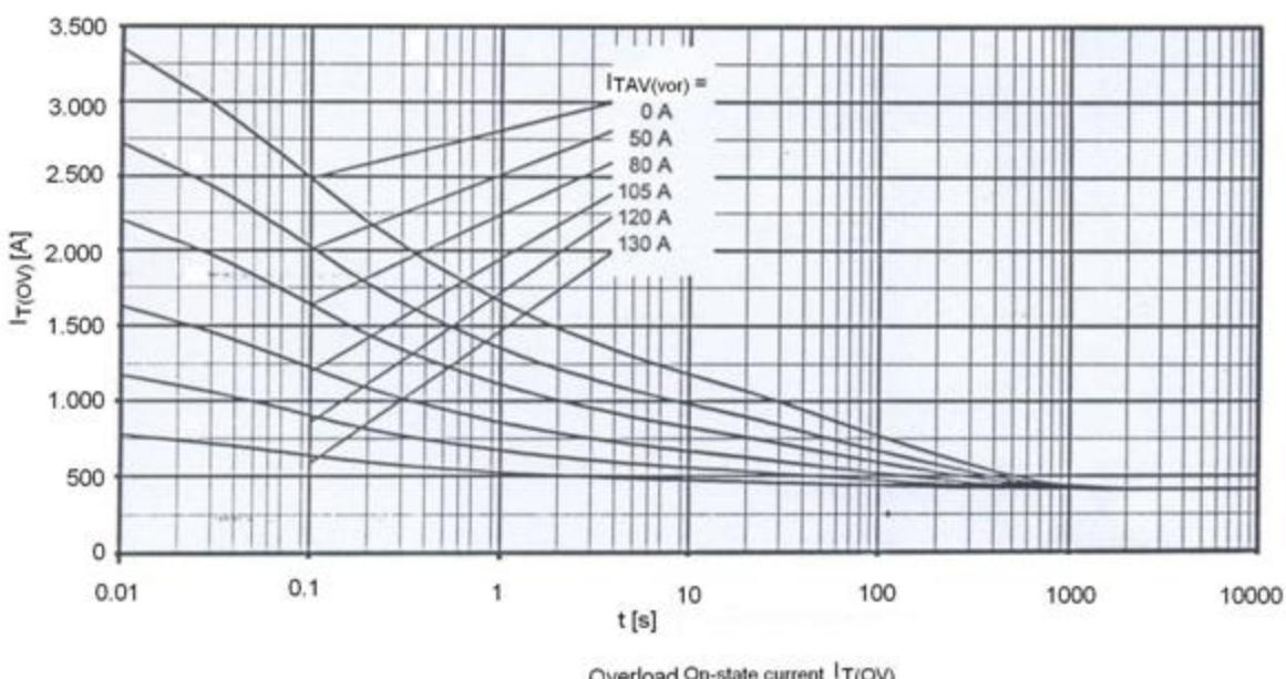
B6- Six-pulse bridge circuit, 120° rectangular
